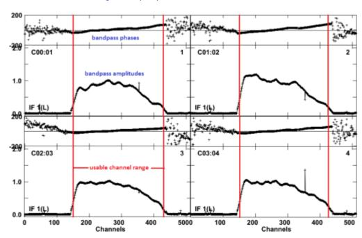
Note down the lower- and upper-limit of the channel range. Then re-run *pre\_calibrate\_targets()* as follows:
